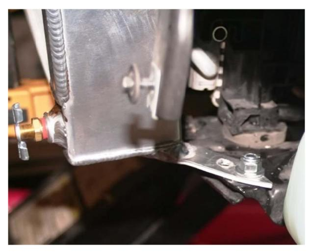
Connect the hoses. Open the petcock. Pour some fresh distilled water/antifreeze into the reservoir to help flush any installation induced debris from the system -  $\frac{1}{2}$
