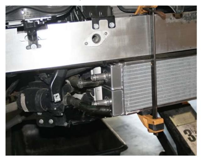
Ensure that the fore-aft location of the new heat exchanger *does not* contact any of the air conditioning equipment that is directly behind.
